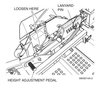
Figure 6-7. Cutter Deck Height Adjustment
